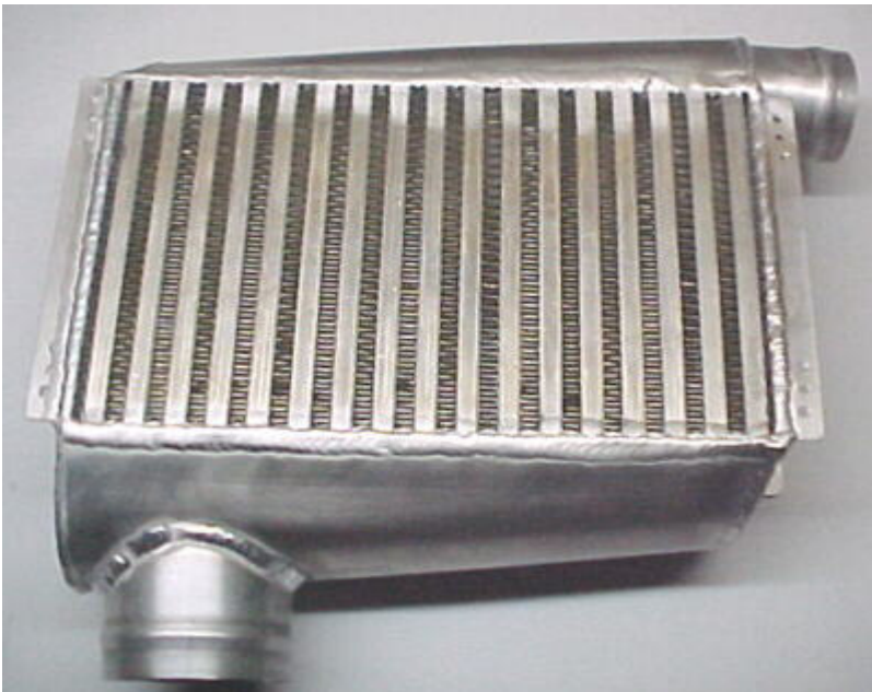
FINISHED INTERCOOLER ASSEMBLY
